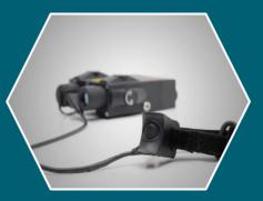
With the dry fire mode it is possible to fire the laser without the microphone by activating the laser with the trigger button. No matter if using a service weapon without blanks or just using a Blue-Gun. The training remains realistic and effective.
