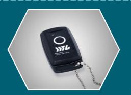
The SIMGUN Respawner is a small sized remote control to reactivate a participant after he got eliminated. Just a short press on the button directly in front of the Body Central Unit sensor and the trainee is back in training.
